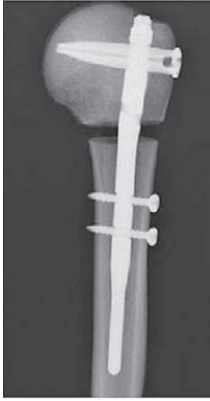
Fig. 1: The Proximal Humeral Nail was used in all specimens, whereas different distal locking-screw mechanisms were used.
