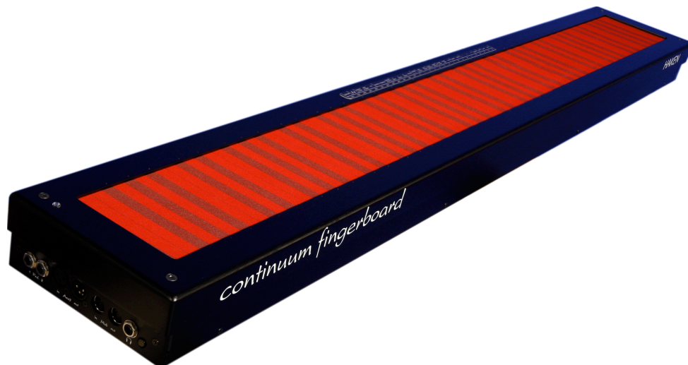
Figure 2.4. The Continuum Fingerboard from Haken Audio has a control surface inspired by the piano. As its name implies, the board enables continuous pitch control over 8 octaves, and a performer can also control the timbre of each struck note by sliding fingers in the so-called y direction (front to back). Photo from http://www.HakenAudio.com/Conituum .
