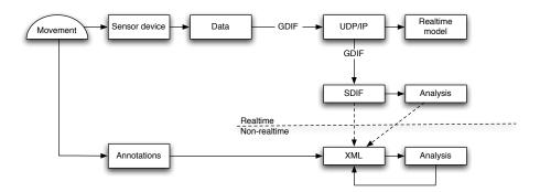
Figure 1: Sketch of data flow for GDIF streaming and storage.
