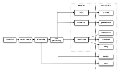
Figure 3: A sketch of how we envisage a multilayered OSC namespace in GDIF.
