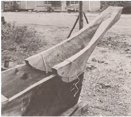
Illustration 11 Wing stem being fitted to the bow of the canoe, from Arima 1975: 144
