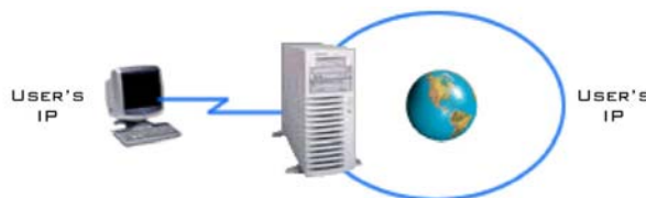
FIGURE 1: STANDARD INTERNET CONNECTION THE IP ADDRESS OF THE USER IS EXPOSED AND EVERY SITE VISITED CAN SEE IT.
