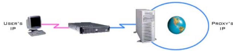
FIGURE 2: PROXY INTERNET CONNECTION THE USER CONNECTS THRU A PROXY SERVER THAT IS CONNECTED TO THE INTERNET. ONLY THE PROXY SERVER'S IP ADDRESS IS REVEALED WHILE THE USER REMAINS ANONYMOUS.
