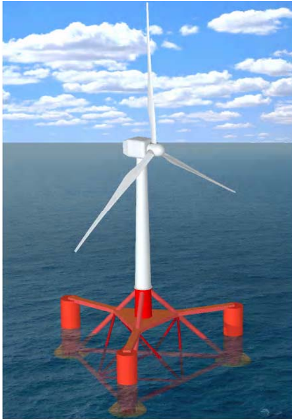
The Triple Floater Concept Source: Bulder et. al. (2003), vi.
