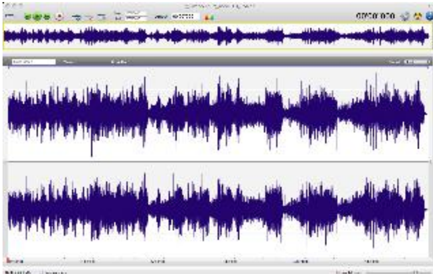
Figure 2. Waveform representation of sound pressure level illustrating the dynamical variations in Brandenburg Concerto No. 3. The x- axis represents time and the y- axis represents sound pressure level (amplitude).
