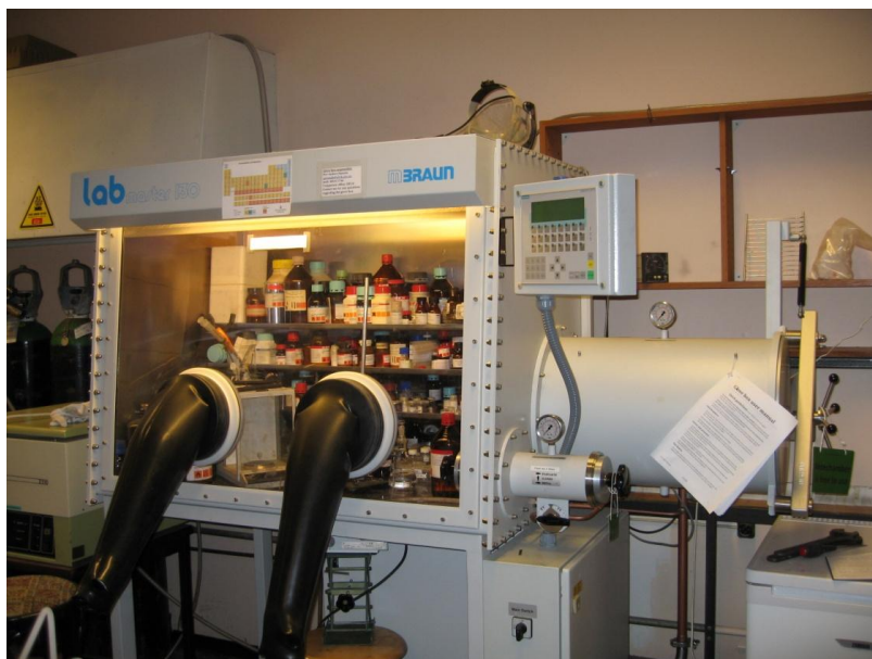
Figure 2-7. A picture of a glove box. The two airlocks can be seen on the right side.
