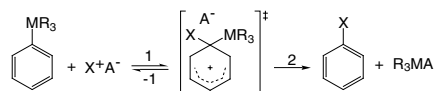
Figure 2.2: Proposed reaction mechanism of the halodemallation using aryltrialkyl group 14 organometallic precursors, from Refs. [14, 24].
