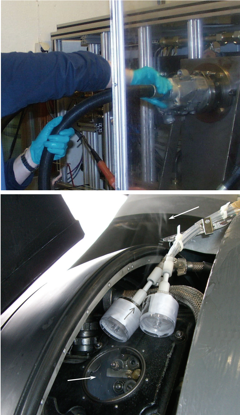
Figure 2-12: Top picture – testing of hydraulic device. Bottom picture – propeller adjustment and visible spray (shown with white arrows) of hydraulic oil from the reservoir
