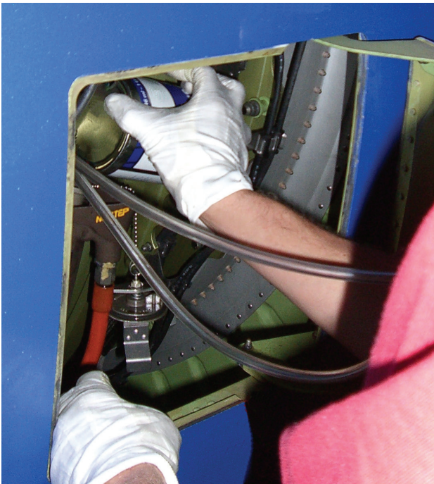
Figure 2-10: Engine maintenance. To the left - airplane engine opened for engine inspection (boroscopy); to the right - draining of jet fuel and oil from aircraft engine.
