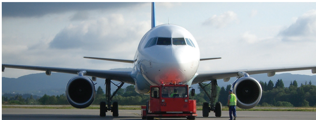
Figure 2-14: Loaders are pushing the aircraft out from the tarmac (push-back)
