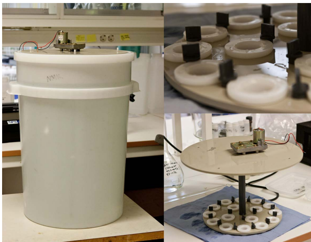
FIGURE 31 Left: 50 L container with motorized lid. Bottom-right: Lid for container with 15 Volt electrical motor on top, for rotating a disk containing P-DGTs. Top-right: P-DGTs fit into apertures and are secured to the rotating disk with twistable clips.
