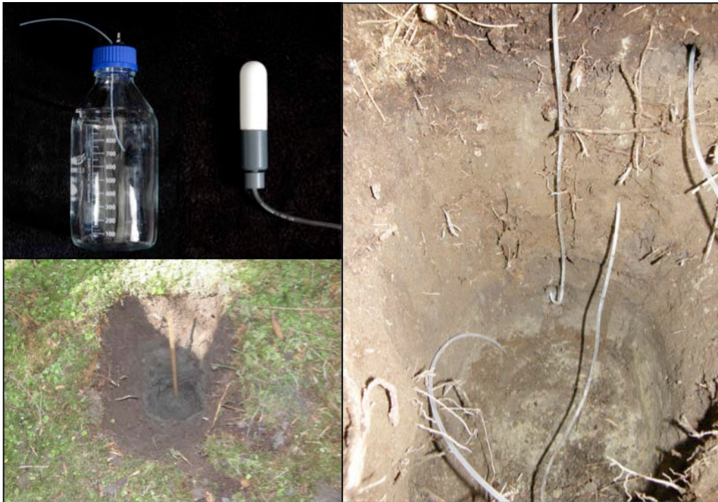
FIGURE 3f Top left: Ceramic lysimeter and 1 L vacuum sampling flask. Bottom left: Photo of dug out hole used to place lysimeters in soil. Right: Photo of lysimeter placed in the different soil horizons.
