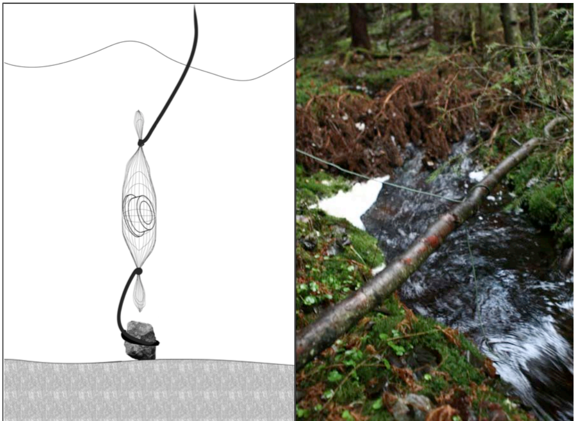
FIGURE 3j Left: Illustration of how the P-DGT is anchored to the stream bed. Right: Photo of Dalen stream, where P-DGTs have been anchored for sampling.
