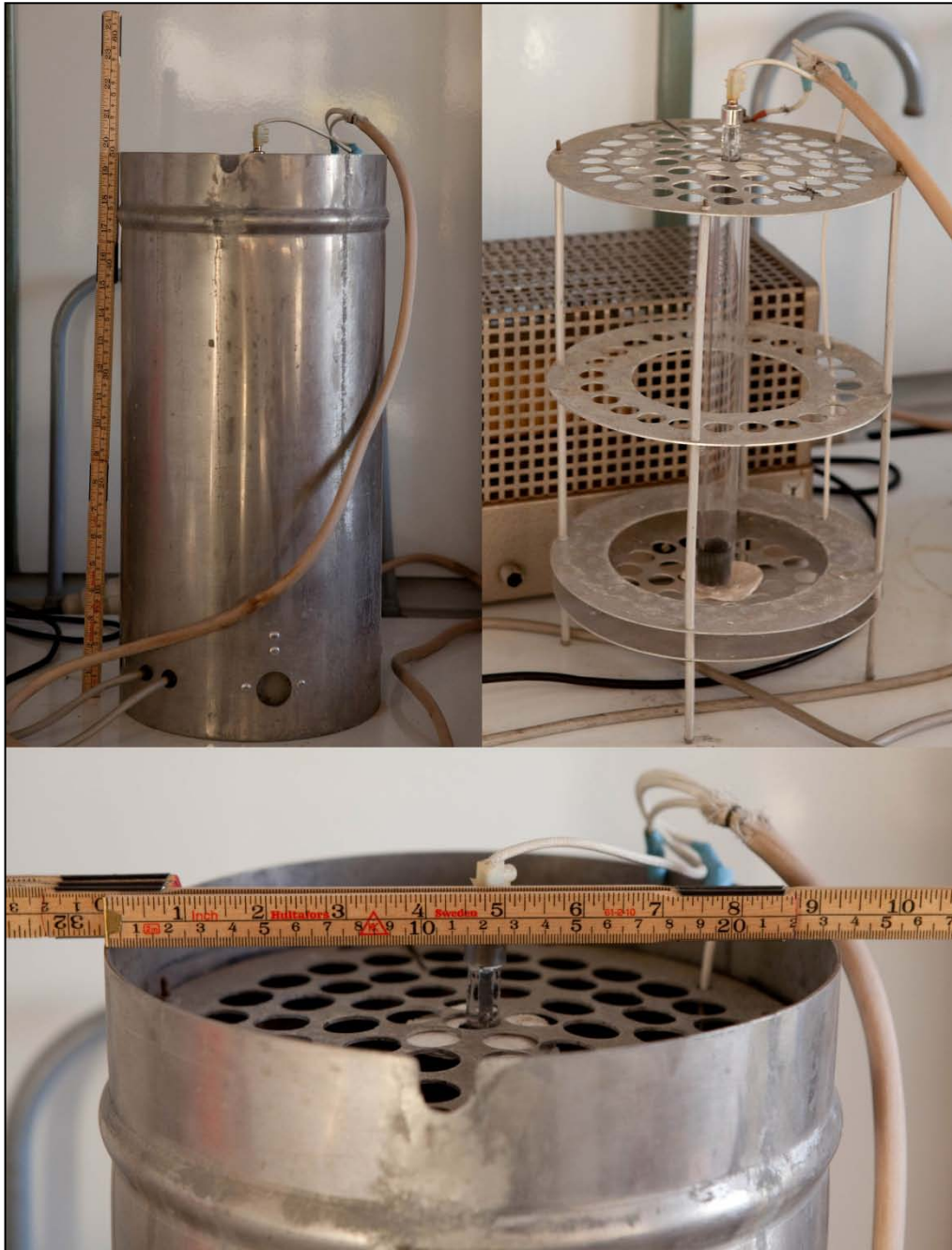
FIGURE 3m Top left: UV-reactor tank approx. 50 cm in height. Top right: Insides of the UV-reactor tank. UV light bulb in the centre, and the quartz tubes with sample are placed around (not shown). Bottom: Top of tank where the quartz tubes are inserted (only in the outer holes. Tubes are approx. 3 cm from the UV light bulb.
