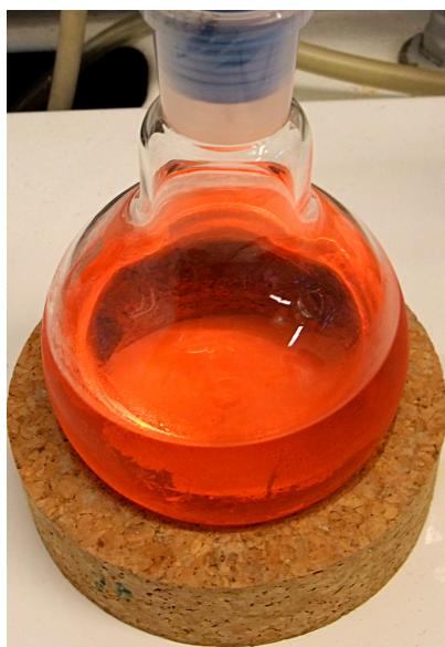
Figure 4.1. – 2 mmoles of 2d undergoing thermolysis. The septum is perforated with a cannula and is only present to avoid evaporation.
