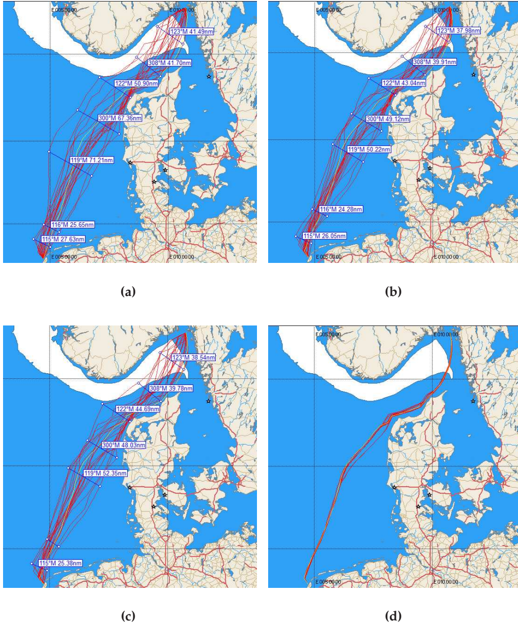
Figure 5.17: Optimal routes for the experiments in the downwind case. In a) Experiment 3DN, in b) Experiment 4DN, in c) Experiment 5DN and in d) Experiment 6DN. The blue lines across the routes and the number boxes indicate the distance across the ensemble of routes. The route given by the yellow line is the path suggested by the control member of the forecast ensemble.
