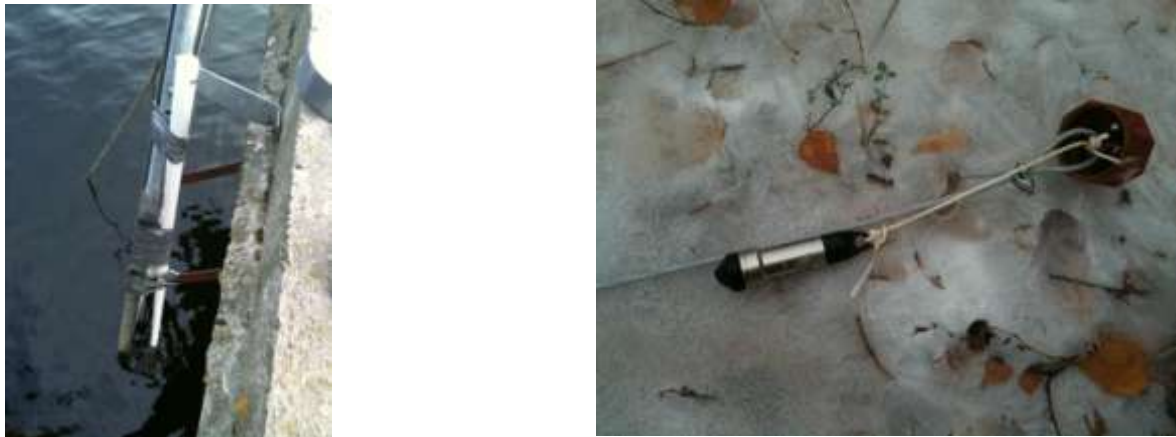
Figure 3.1.2 Tide observation point and the GR02 barometric observation device
