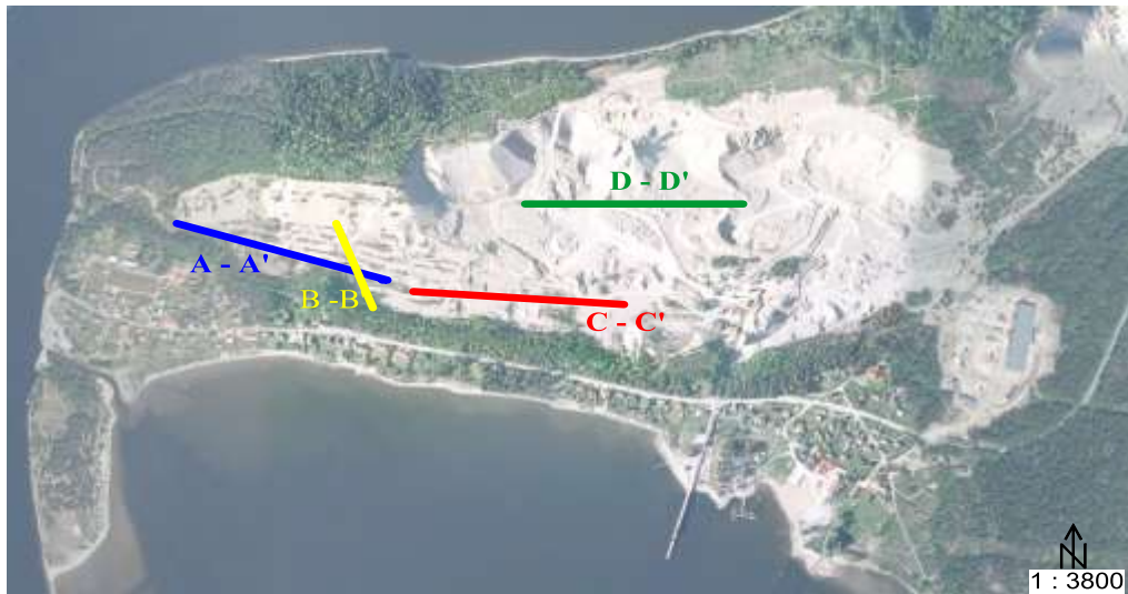
Figure 3.2.5 Location of the resistivity lines
