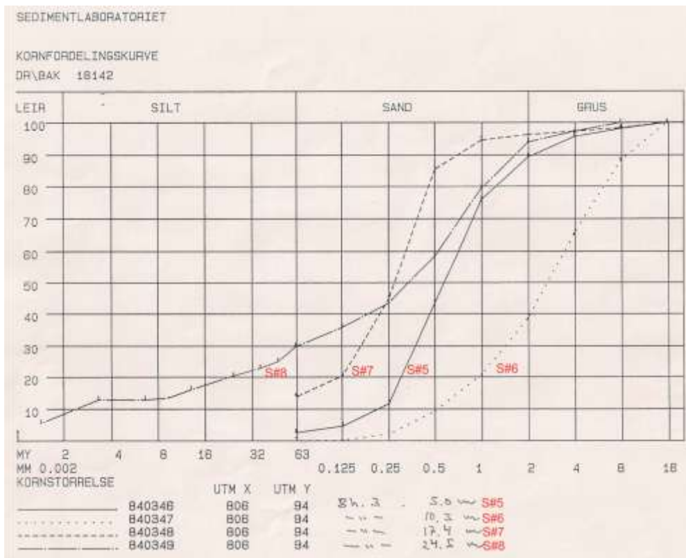
Figure 4.1.3 Grain size distribution from BH3
