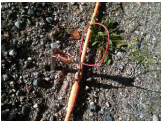
Figure 3.2.3 Electrode in ground
