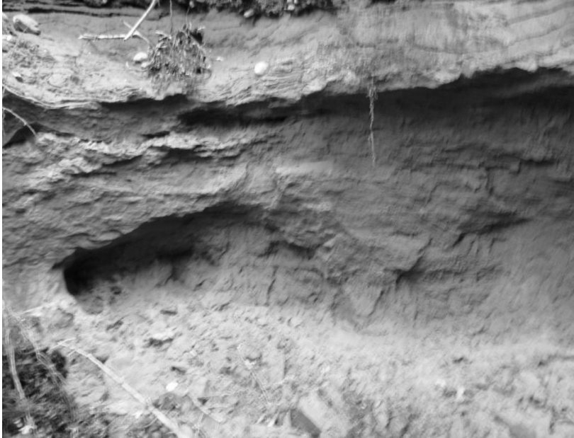
Figure 3.2: Rear part of the avalanche pit 1 with sand layer at the bottom
