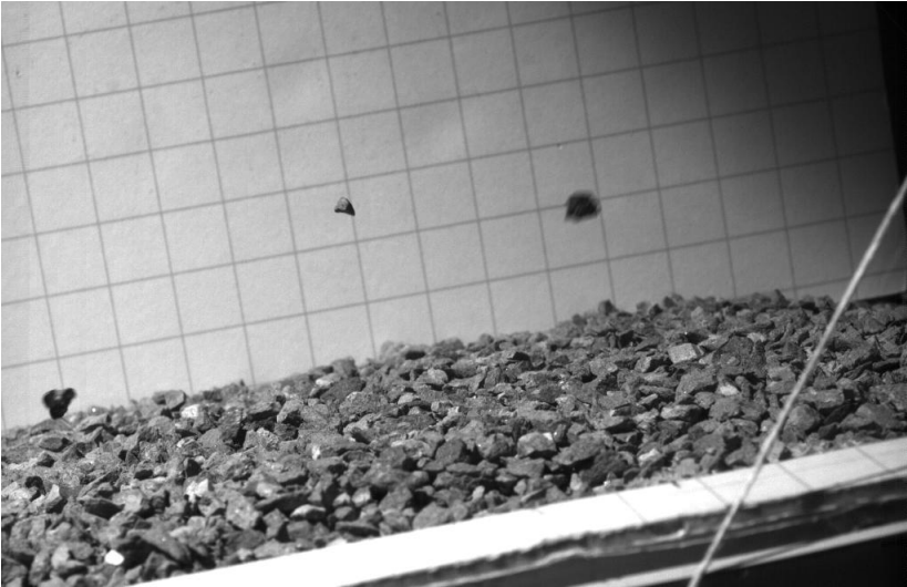
Figure 7-46 Fall and bouncing of spherical pebbles.
