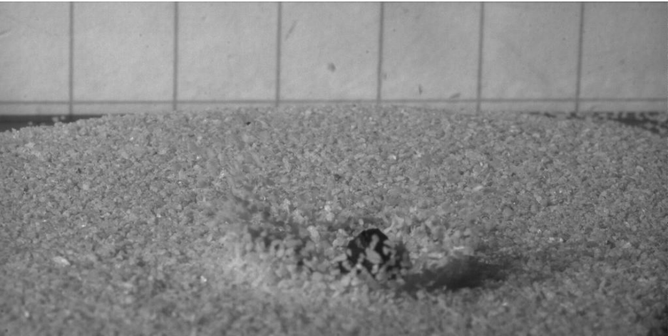
Figure 0-14 Impact of spherical pebble falling on flat yellow coarse sand bed. Grains bounce 0, dive and stop. Bed grains bounce a lot and above measured area. Velocities of grains after impact is estimated from 0 m/s to 0,31 m/s. With height of fall of 60 centimetres the velocity before impact is 3,431 m/s. The calculated coefficient of restitution from 0 to 0,09.
