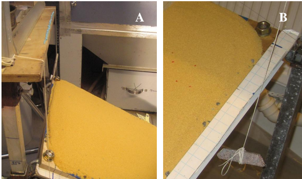
Figure 5-2 A. Experimental set-up for exploring the run-out and distribution of grains. B. Lead line from the height adjustable board.
