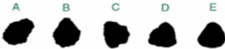
Figure 4-2 Pettijohns (1957) description of roundness. A: Angular. B. Subangular. C. Rounded. D. Subrounded. E. Well rounded (Bjørlykke, 1977).
