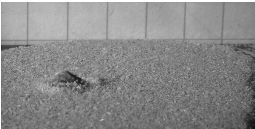
Figure 0-11 Impact of flat pebble falling on flat yellow coarse sand bed.
