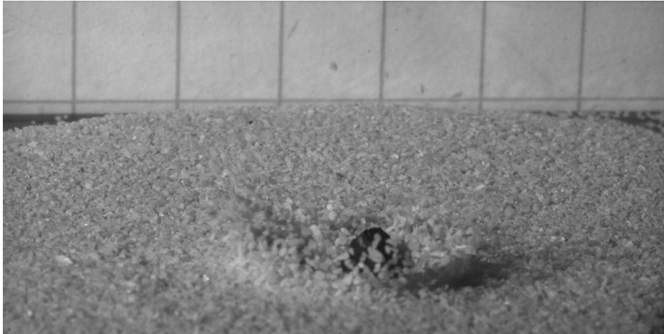
Figure 7-5 Impact of spherical pebble falling on flat yellow coarse sand bed.
