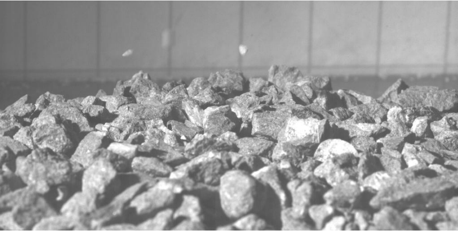
Figure 0-102 Impact and bouncing of red very coarse sand on flat pebble bed.
