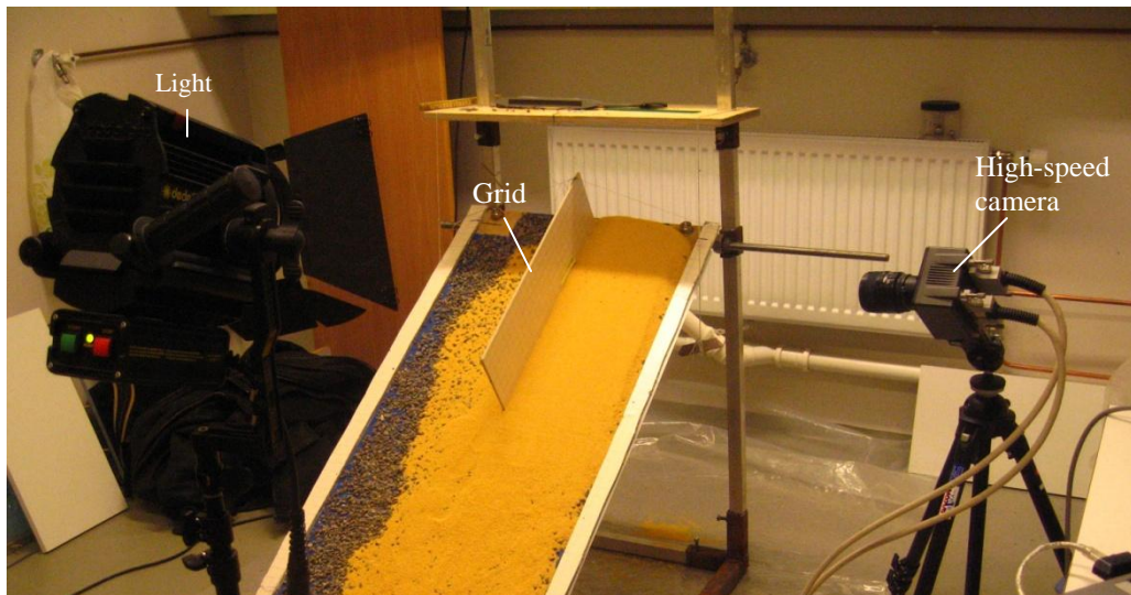
Figure 7-1 Experimental set-up for capturing of particle motion at impact by use of high-speed camera
