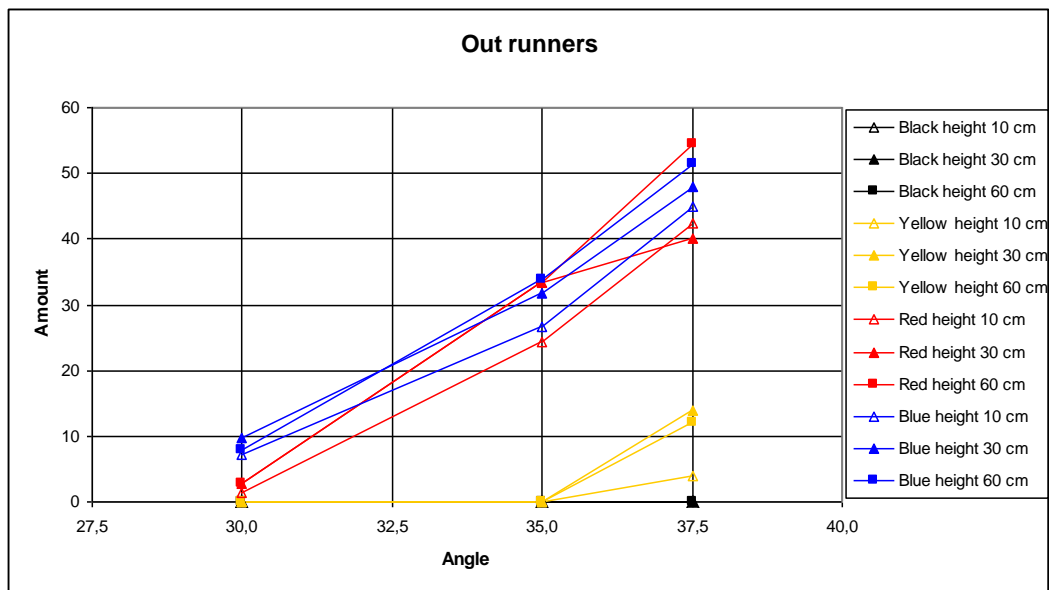
Figure 5-33 Amount out-runners for all grain sizes, fall heights and slope angles used in the experiments.
