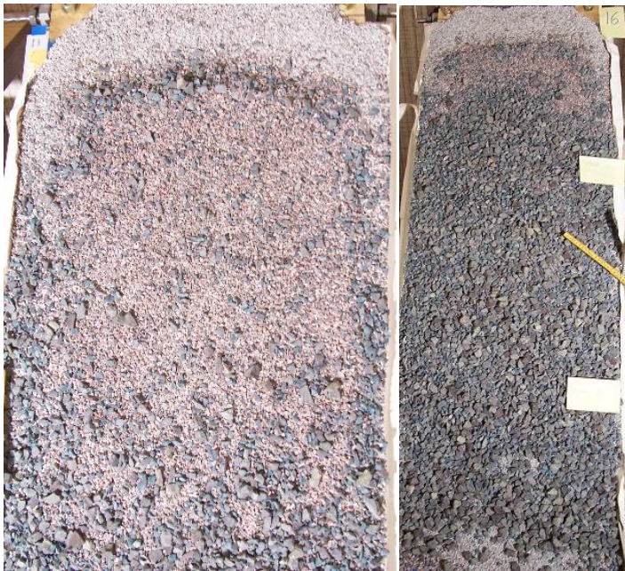
Figure 8-3 A sequence taken from the experiment. A: at the beginning of the experiment, small particles stay close to the fall zone, while many of the large ones are capable to roll down to the slope break. B: After five sub-runs, a clear distribution of particle size increasing down slope ensues, except for a zone still devoid of new particles (the white bed is formed of small-size particles that have been placed on the table from the beginning of the experiment). C: Slide scar after a major failure at the top of the artificial talus. Note that the only visible particles are the small ones. D: At sub-run 16, the slide scar begins to be filled by the newly falling particles, to form a new accumulation that may eventually slide again.
