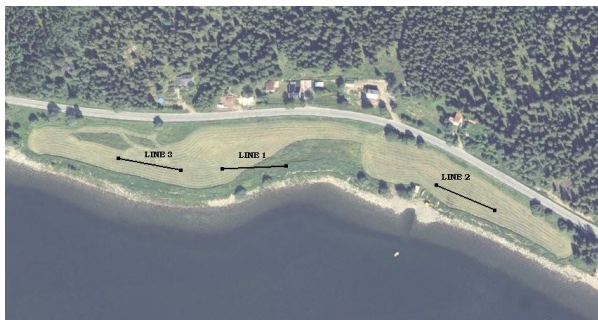
Figure 3.4 An overview on the investigation area with the three seismic lines displayed. Line 1 in the middle, line 2 in the eastern part and line 3 in the western part of the area. Each seismic line is 46 m long. The main road in the area with local houses located north of the investigation area. Background photo from www.norgebilder.no .
