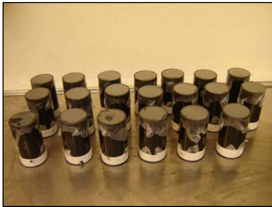
S/S contaminated sediments
