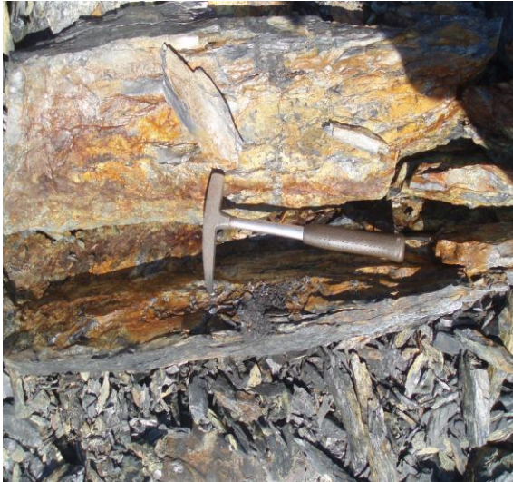
Figure 4-29 Inside of one alum shale rock split into two where the hammer placed. The reddish brown color is due to iron oxide
