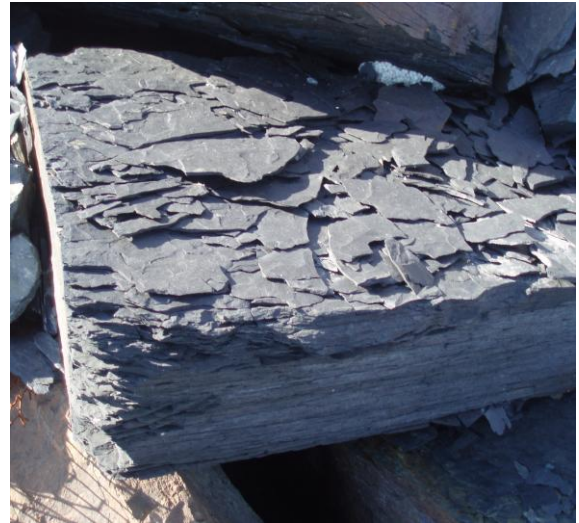
Figure 3-2 Slemmestad Black shale rock placed on an embankment of the sea, were fractured into small pieces
