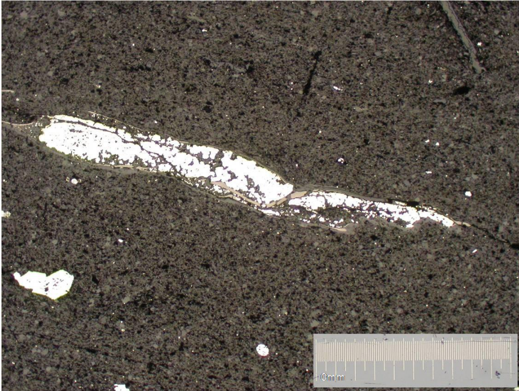
Figure C-7 Tectonized “fish” of recrystallized pyrite (with chalcopyrite) rimmed with recrystallized coarse graphite. X5 BS
