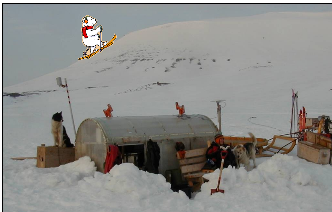
Figure 3.1 The observation hut, "Chalet de Ulli", set up 1 km east of Bogerbreen. The temperature sensor T2 is visible at the pole on the left of the hut. View towards south east during midnight.
