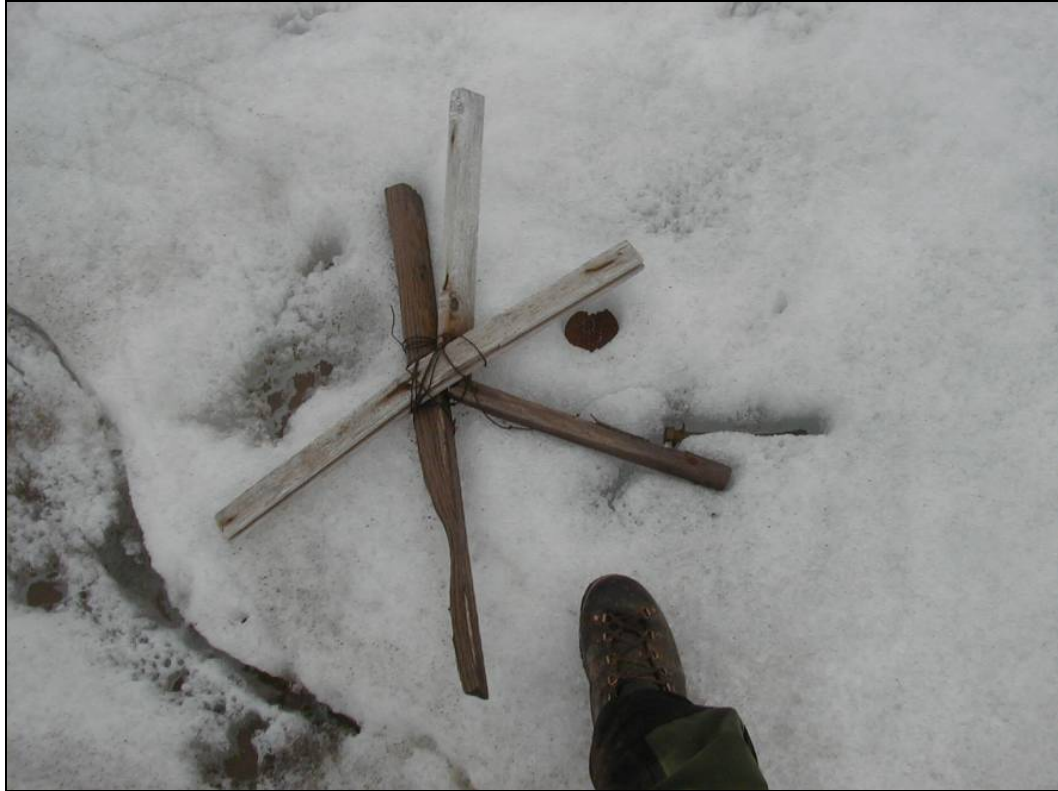
Figure 5.13 Tetrahedron, cable, weight and the marker of the installation to measure glacier surface ablation. Such installations were found on several locations during a field visit on 12 th of August 2005.
