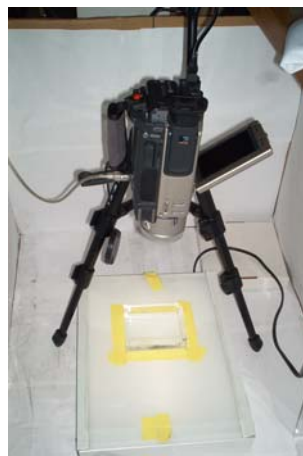
Fig. 2.1. The video record setup , including the plexi glass view tray on a light box. All housed in a large cardboard box in order to avoid the fry getting disturbed by external activities.
