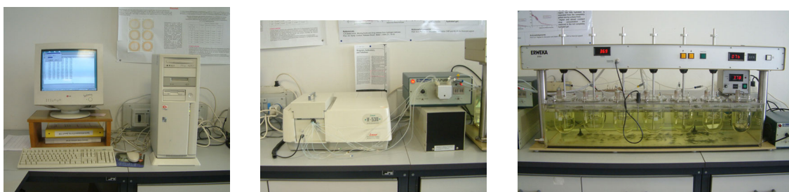
Figure 17: The computer, spectrophotometer, pump and paddle apparatus used during the dissolution.
