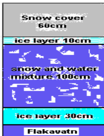
Figure 3.2: Flakevatn winter 2004/2005 ice/snow cover vertical profile. The profile shows interchanging layers of snow, ice and ice/water slurry. 40cm of ice is a more accurate estimate than Strøm 1965 150cm thick ice.
