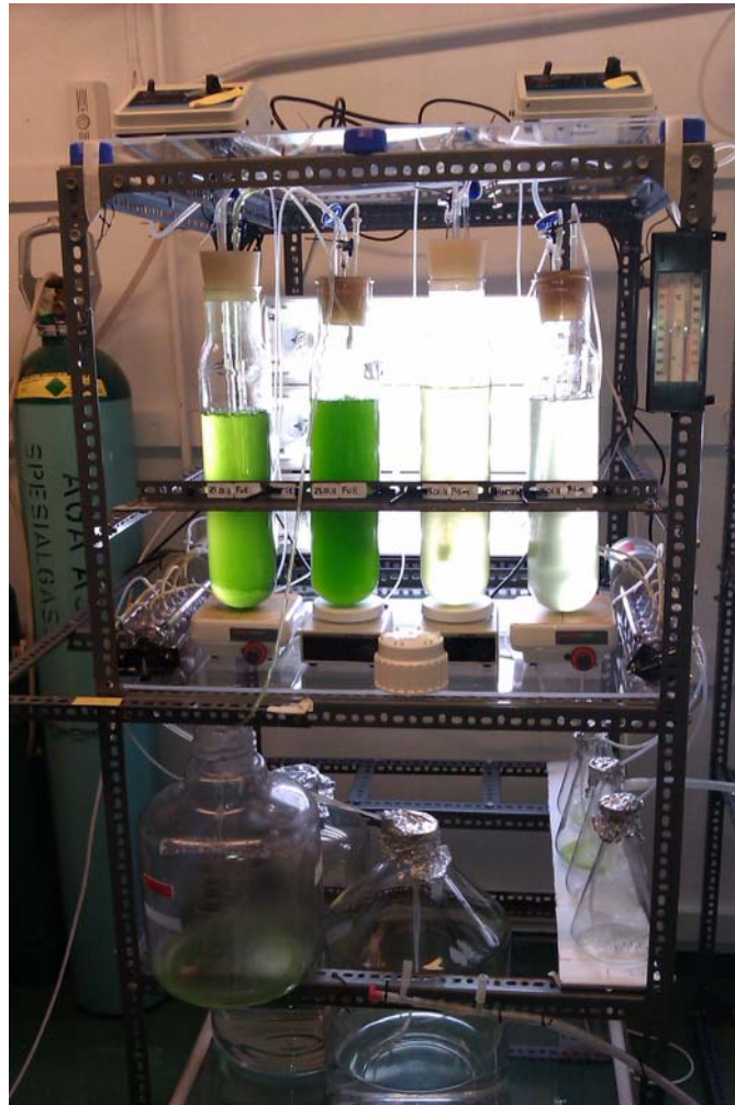
Figure 4: Chemostats system with four glass tubes that were used throughout all experiments, two with full medium (left) and two with P limited (right). Full chemostats characterize with higher algal density and dark green color while less dense P limited algae have a yellowish green color. This results in different extinction coefficient for different chemostats.
