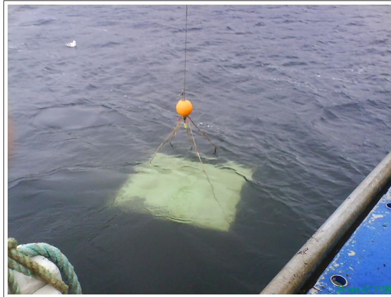
Figure 2.3: Picture of the recapturing of one of the frames from the bottom at the experimental site. Each frame had a curtain with a mechanism that closed the curtain when the frame was pulled up from the bottom. The function of the curtain is to make sure that the material stays in place. Photo: Frode Olsgard with permission
