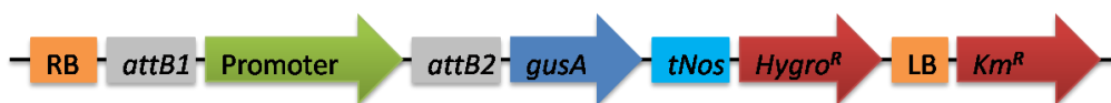
Figure 2.2 The GUS construct. The inserted promoter region is flanked by attB sites (25 bp) and followed by the coding sequence (CDS) of gusA , encoding the \beta -glucuronidase. RB: Right border, LB: Left border, tNos : Nos terminator, Hygro R : Hygromycin resistance gene, Km R : Kanamycin resistance gene ( NptII ). The figure is not to scale.
