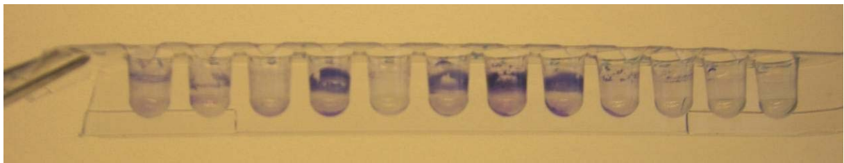
Picture 3.7: Biofilm ring formation for biofilm-positive (+) and biofilm-negative (-) strains, after 72 hours incubation. Left to right; AH75 (+), AH604 (+), AH226 (+), AH405 (+), AH183 (-), AH815 (+), AH884 (+), AH1031 (+), AH1248 (-), AH1271 (-), AH1353 (-) and negative control (pure bactopectone medium).
