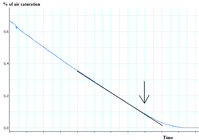
Figure 7. Example of recording of falling oxygen-levels in water during closed respirometry. When oxygen concentration decreases below the critical oxygen tension ( [O_2]_{crit} , arrow), the fish will no longer take up oxygen at a constant rate.
