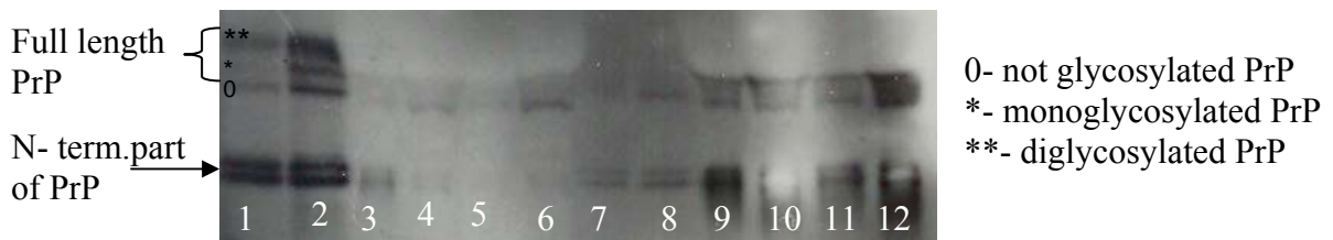
Figure 34: Western blot of immunoprecipitation, anti-PrP P4 (1:10000) and anti-mouse true blot (1:100) were used as primary and secondary antibodies, respectively: 1) PrP-EGFP IP P4; 2) PrP-EGFP-PINT IP P4; 3-4) PrP-EGFP and PrP-EGFP-PINT lysates after IP with P4, respectively; 5-6) PrP-EGFP and PrP-EGFP-PINT lysates before IP with P4, respectively; 7) PrP-EGFP IP anti-RFP; 8) PrP-EGFP-PINT IP anti-RFP; 9- 10) PrP-EGFP and PrP-EGFP-PINT lysates after IP with anti-RFP, respectively; 11- 12) PrP-EGFP and PrP-EGFP-PINT lysates before IP with anti-RFP, respectively; 12% acrylamide gel.
