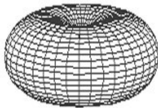
Figure 2.16: Emission diagram of a short dipole takes the form of a torus
