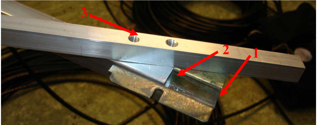
Figure 3.2: Bottom- side picture of the top attachment piece (1), the rear end of the front antenna boom (2) and the custom made aluminium piece with screw-holes (3).
