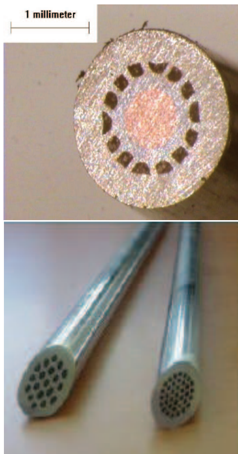
Fig. 1.1: Superconducting wire based on \text{MgB}_2 . Black dots in the wire are \text{MgB}_2 itself, the rest is Cu surroundings. Maximum current of the wire at 27.5K – 330A. Standard batch length: in 2005 year - 1.6km, in 2006 year - 7km. Taken from site of COLUMBUS SUPERCONDUCTORS SPA ( www.columbussuperconductors.com ).
