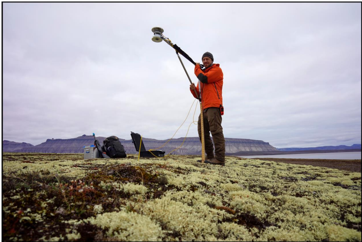
Fig. 6: Albedo measurements on Flinholmen, Svalbard. Research collaborator Rasmus Erlandsson, Norwegian Institute for Nature Research, controls that the albedometer instrument is stable.
