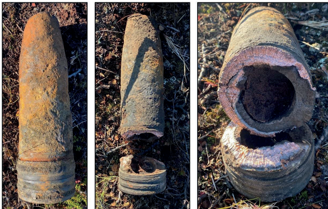
Fig. 2. A German 88 mm HE projectile (type 8.8 cm Sprgr. Patr. L/4.5 (Kz)) cut with a flexible linear-shaped charge. Its filling is identified as Füllpulver 60/40 (i.e., Amatol 40/60).
