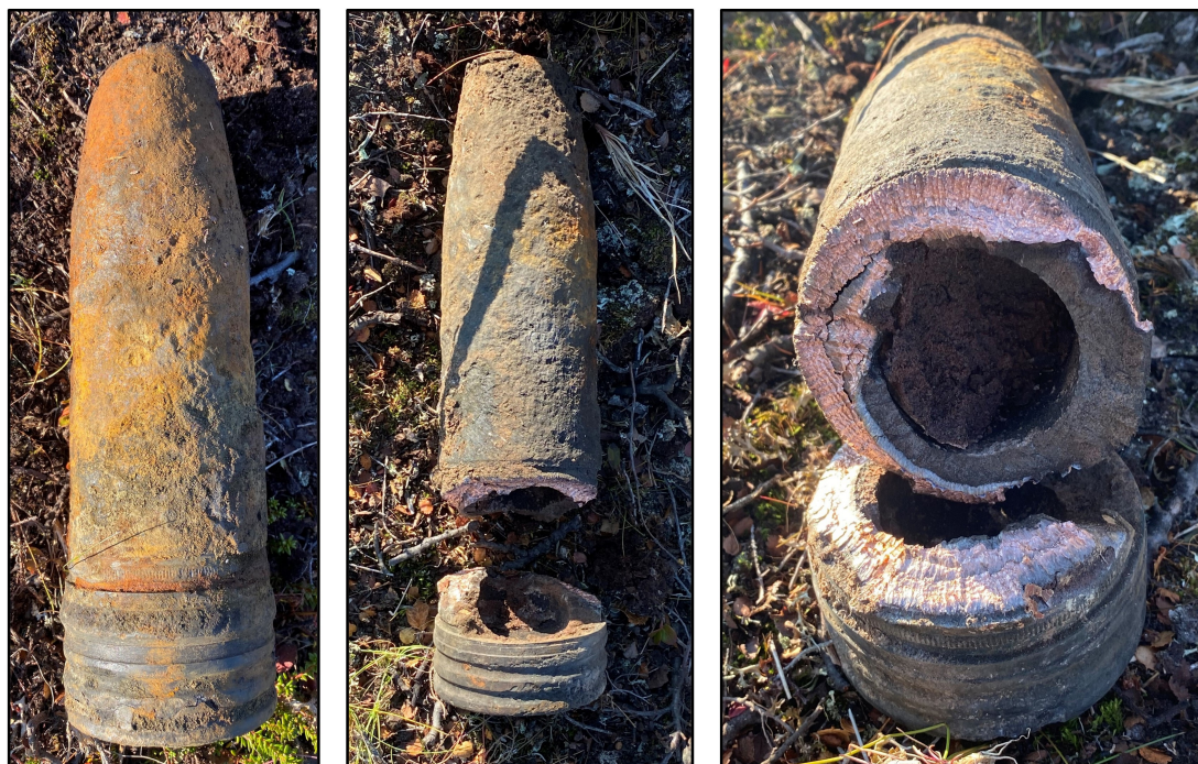
Figure 2. A German 88 mm HE projectile (type 8.8 cm Sprgr. Patr. L/4.5 (Kz)) cut with a flexible linear-shaped charge. Its filling was identified as Füllpulver 60/40 (i.e. Amatol 40/60).
