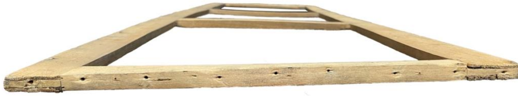
Fig. 6 The strainer after removal of the painting, showing distinct warping.
