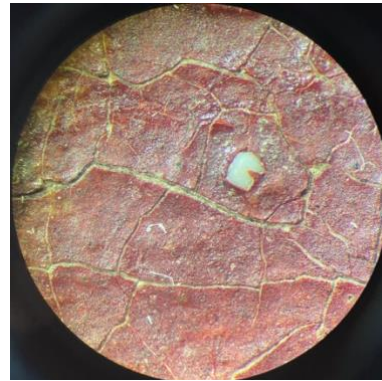
Fig. 11 Example of a single metal soap protrusion in the paint layer. Many such protrusions were found.
