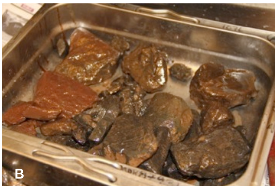
Figure 6. (A) FP2 fractures with carbonate fracture fill. Also note oxidised haloes along fractures. This fracture population is only found intraformationally in siltstone stringers in the upper part of the Draupne Formation. (B) Rubble zone in siltstone layer, which was probably generated by drilling-induced collapse of the FP2 fracture system.
