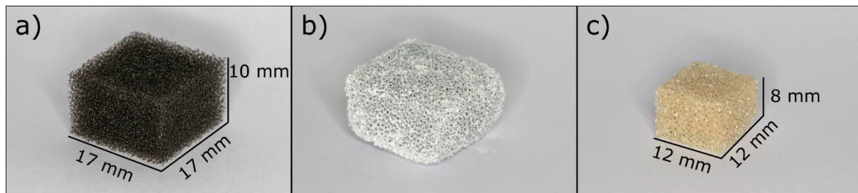
Figure 5- Scaffold production. a) Original foam template, b) Coating of foam template with a TiO 2 slurry, c) Final scaffold. Note shrinkage of the ceramic following sintering.
