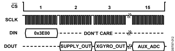
Figure 12. Burst Read Sequence
