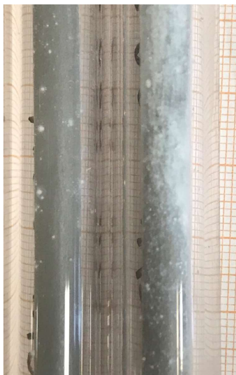
Figure 29: Monel crucibles covered in fibrous quartz after attempted oxyfluoride synthesis. The left and right crucibles correspond to “ZnOF” and “Co 10 O 4 F 15 ” syntheses, respectively.
