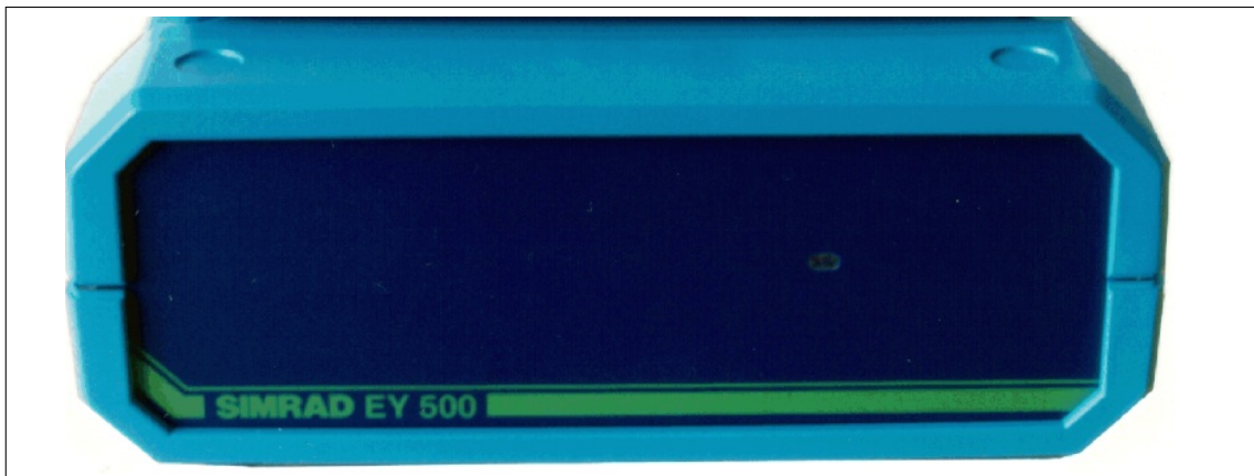
Figure 4.1: Image of the Simrad EY500 transceiver unit taken from the Instruction Manual. The unit is considerably larger than the prototype circuit board designed in the project.
