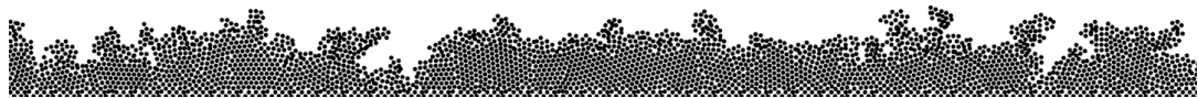
Figure 7.20: Final surface created by linear gradient percolation and the random drop method with \zeta = 1/3 .
