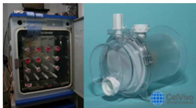
Figure 6. Rotary cell culture system from CelVivo used to produce spheroids (255).
