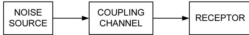
Figure 5.9: Typical noise path. All three blocks must be successfully identified to analyze a noise problem.
