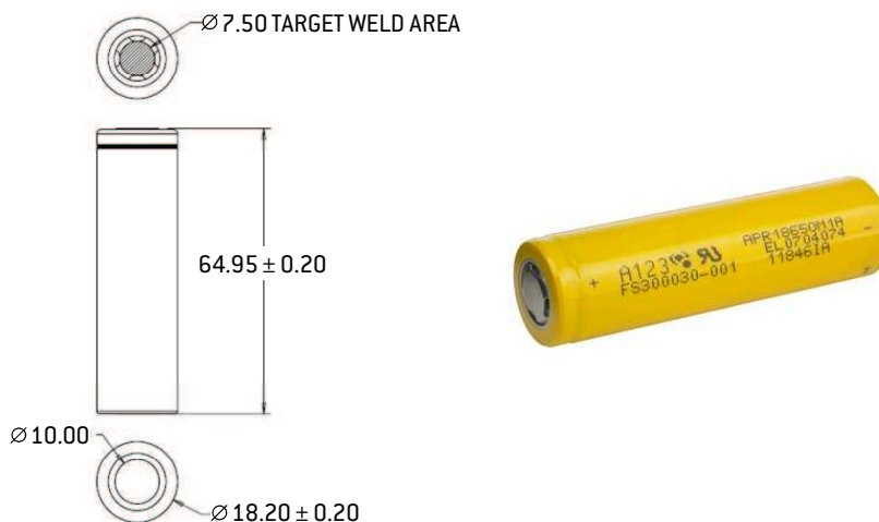
Figure 3.9: A123 Systems LiFePO 4 cell dimensions and picture.
