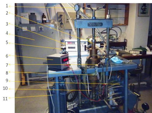
Figure 4.2: Synthesis: sintering instrument. 1- dimension detector; 2- lid; 3- programming; 4- supply current; 5- pressure gauge; 6- thermometer; 7- thermocouple; 8- furnace; 9- cooling water; 10- forcing press, 11- oil pump.
