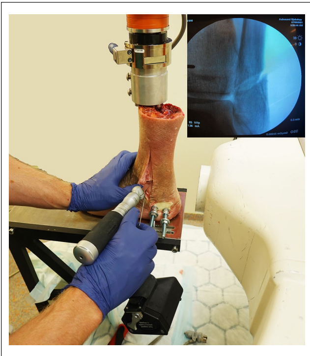
Figure 2. Depiction of how oblique, transsyndesmodic fibula osteotomies were made.
