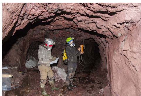
Figure 4. Photo of one locality, showing alpha track detectors as hung from the roof and the position of the GEORADIS gamma spectrometer.
