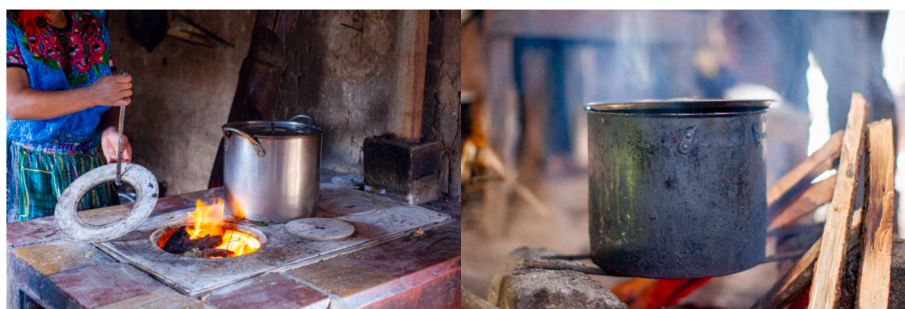
Fig. 1. The left image depicts the Plancha chimney intervention stove in San Lorenzo, Guatemala. Fuel is fed into an enclosed combustion chamber (not visible); smoke vents out through a chimney (near the rear of the stove). The right image depicts a typical open fire cookstove.
