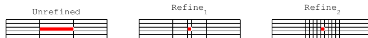
Figure 6.9: Refinement of the column of the grid containing a well-block. The well-block is colored.
