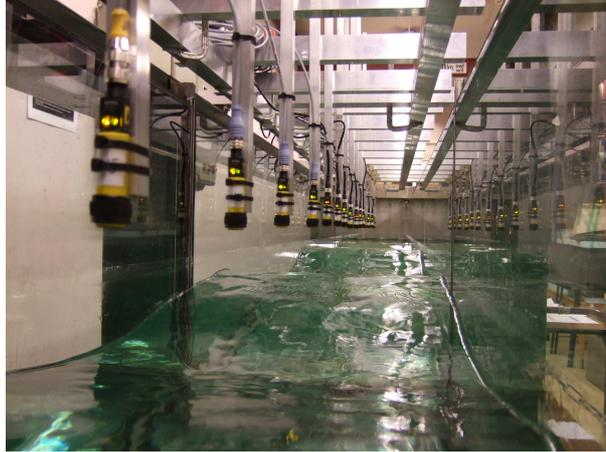
**Figure 4:** The linear array, wave generator (end) and the wave field.
