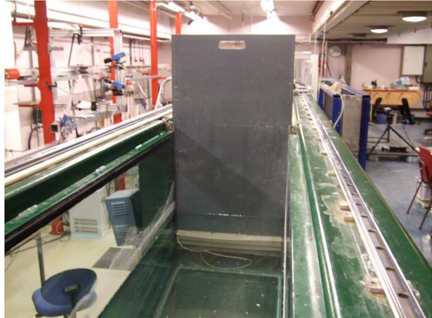
Figure 59: Reflecting wall.
