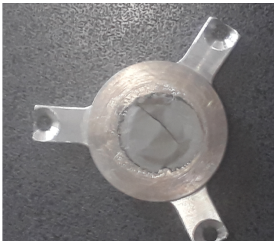
Figure 4.11: One of the thin ^{124}\text{Sn} targets, that was mounted and stretched onto a plunger frame, but later broke.
